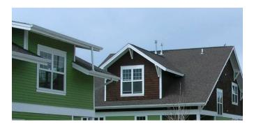
• Shed dormers shall have a pitch of at least 3:12. Hip and gable dormers shall have the same pitch as the main roof volume.
